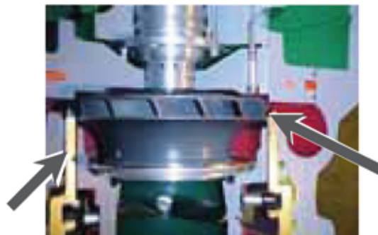
Figure 2: Movable diffuser closes impeller discharge area as load decreases.
