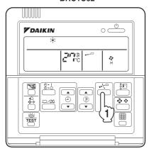
1. Press the AIR FLOW DIRECTION ADJUST button to select the air direction as shown below.
