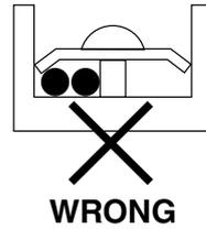
Do not connect wires of different gauges. (WRONG)
