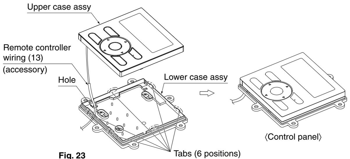
**2. Remove the front panel, and then remove the back plate attached to the back side.**
